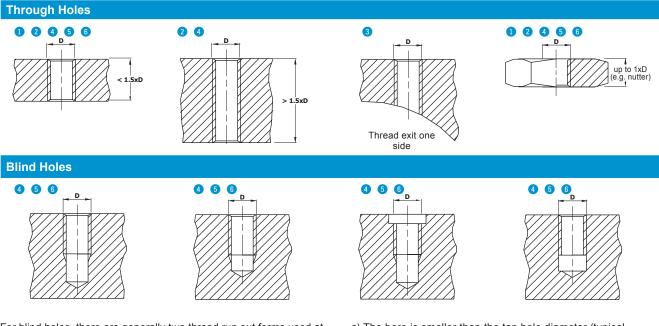
For blind holes, there are generally two thread run out forms used at the bottom of the tap hole. One form has a recessed diameter at the bottom of the hole, and the other form has a standard run out. Other types of holes are respective to construction designs, eg.
