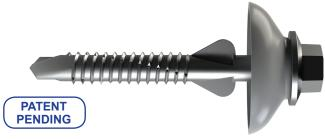
One Step fastening of corrugated and square rib sheeting. Ideal for profile rib heights 16mm to 29mm. Cutting fins automatically form expansion hole and self centre screw during installation. Vortex<sup>™</sup> universal screw for timber or steel up to 1.5mm thick. Armour Coat™ protection to AS 3566 Class 4. 26mm diameter EPDM sealing washer for water tight seal. Available in 50mm and 65mm length.
