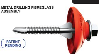
One Step fastening of corrugated and square rib sheeting. Suitable for profile rib heights 16mm to 35mm into steel purlins up to 2.4mm. Cutting fins automatically form expansion hole and self centre screw. Armour Coat™ protection. Weather seal sealing washer for water tight and secure fastening. Hi Visibility seal highlights non trafficable sky light zones. Available in 65mm length.
