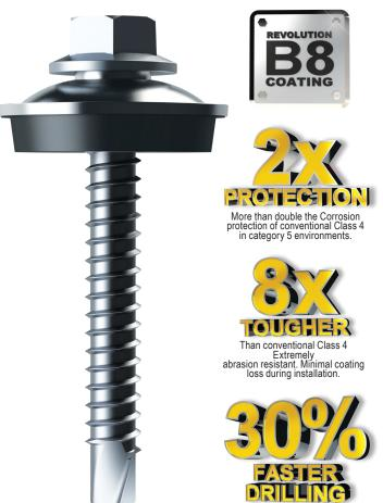
The Bremick Vortex™ Cyclone is a preassembled Universal Cyclone Assembly complete with a marine grade Aluminium/ EPDM "BRA" Cyclone washer, suitable for use with all corrugated and square rib roofing profiles which is mounted on the Vortex™ self drilling screw, designed for universal application into Timber, Metal Battens and Steel purlins up to 2mm thick.\* Available in 25mm, 55mm, 65mm and 95mm.
