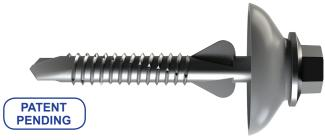
One Step fastening of corrugated and square rib sheeting. Ideal for profile rib heights 16mm to 29mm. Cutting fins automatically form expansion hole and self centre screw during installation. Vortex™ universal screw for timber or steel up to 1.5mm thick. Armour Coat™ protection to AS 3566 Class 4. 26mm diameter EPDM sealing washer for water tight seal. Available in 50mm and 65mm length.
