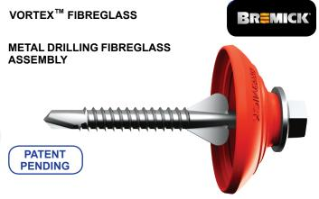
One Step fastening of corrugated and square rib sheeting. Suitable for profile rib heights 16mm to 35mm into steel purlins up to 2.4mm. Cutting fins automatically form expansion hole and self centre screw. Armour Coat<sup>™</sup> protection. Weather seal sealing washer for water tight and secure fastening. Hi Visibility seal highlights non trafficable sky light zones. Available in 65mm length.
