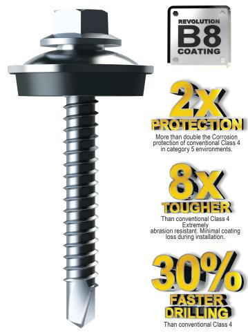
The Bremick Vortex<sup>™</sup> Cyclone is a preassembled Universal Cyclone Assembly complete with a marine grade Aluminium/ EPDM "BRA" Cyclone washer, suitable for use with all corrugated and square rib roofing profiles which is mounted on the Vortex<sup>™</sup> self drilling screw, designed for universal application into Timber, Metal Battens and Steel purlins up to 2mm thick.\* Available in 25mm, 55mm, 65mm and 95mm.
