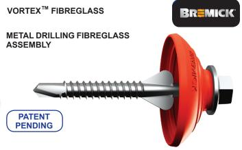
One Step fastening of corrugated and square rib sheeting. Suitable for profile rib heights 16mm to 35mm into steel purlins up to 2.4mm. Cutting fins automatically form expansion hole and self centre screw. Armour Coat<sup>™</sup> protection. Weather seal sealing washer for water tight and secure fastening. Hi Visibility seal highlights non trafficable sky light zones. Available in 65mm length.
