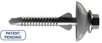
One Step fastening of corrugated and square rib sheeting. Ideal for profile rib heights 16mm to 29mm. Cutting fins automatically form expansion hole and self centre screw during installation. Vortex<sup>™</sup> universal screw for timber or steel up to 1.5mm thick. Armour Coat<sup>™</sup> protection to AS 3566 Class 4. 26mm diameter EPDM sealing washer for water tight seal. Available in 50mm and 65mm length.
